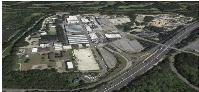
**CHALLENGE:** Care would need to be taken as works would continue around live services such as water, electricity, telecoms and gas. Being an ex-MOD site, there could be a risk of unexploded ordnance (UXOs) buried in the ground. Licensed asbestos was identified in multiple buildings, so this would need removing subject to a Plan of Works for each unit.
