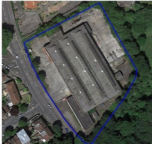
The main structure comprised of a large open space with several inspection pits, several smaller internal rooms were located to the rear of the building. The roof was formed with three pitched sections comprising of a steel frame enclosed with cement bonded roof sheets.
